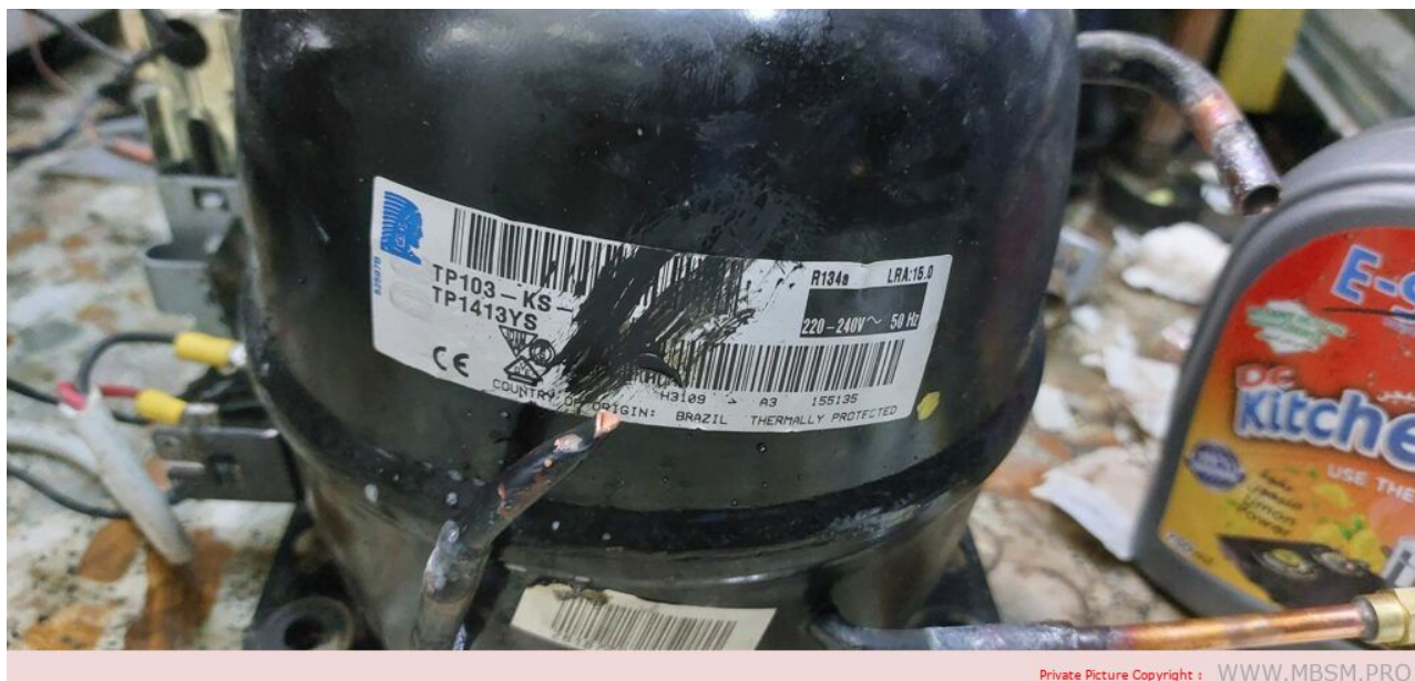
Mbsm.pro, COMPRESSOR, TECUMSEH, 1/3 hp , TP1413YS, R-134A, 220V, lbp
