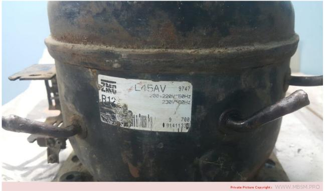
Mbsm.pro, Compressor, Electrolux Group, Zem, Compressor, L45AV, R12, 1/8 hp, HMBP
