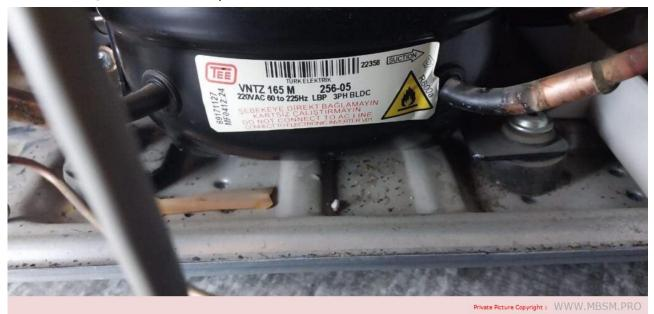
Mbsm.pro, Beko, Compressor, VNTZ165M, VNTZ165MT / VNTZ165M, Tee compressor, R600A, inverter, Blcd, 1/3 hp, lbp, Turk compressor
