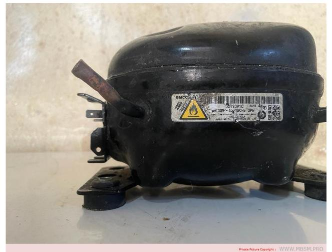
Mbsm.pro, compressors, DZ120V1A, DZ120V1V, DZ120V1B, inverter, blcd, from 1320 to 4320 rpm, from 82 to 265 w input, cooling 293 btu to 904 , 1/3 hp, r600a, lbp
