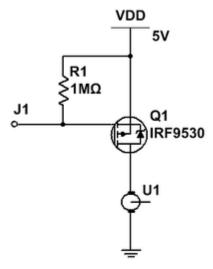
Motor connected from transistor to -V/GND
