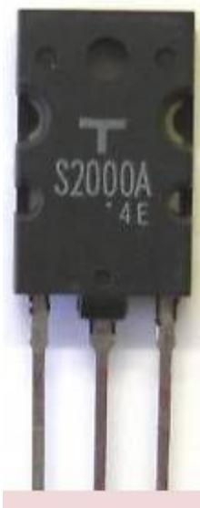
the S2000 is a silicon NPN transistor, Ucb = 1500V, Ic = 8A,
