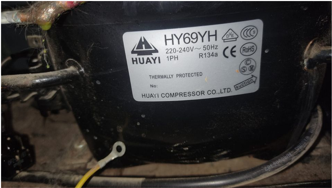
HUAYI, Refrigeration Compressor ,HYE69Y63,R134A, LBP, 195W, 1/5Hp , RSIR,
