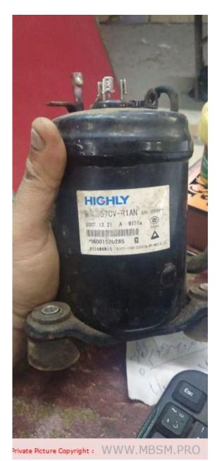
Mbsm.pro, Compressor, bsa357cv-rlan, Highly, Hitachi, R134a, Rotary Compressor, for Air Condition, 220/240V, 1245BTU, run capacitor 5 mF/38, replaced by qx36h
