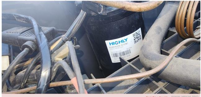
Mbsm.pro, Compressor, HIGHLY, BSA645CR-R1EN, GBSA645CR, 840w, r134a, 1.12hp, Constant-Speed, [1ph] 100/100-110V 50/60Hz
