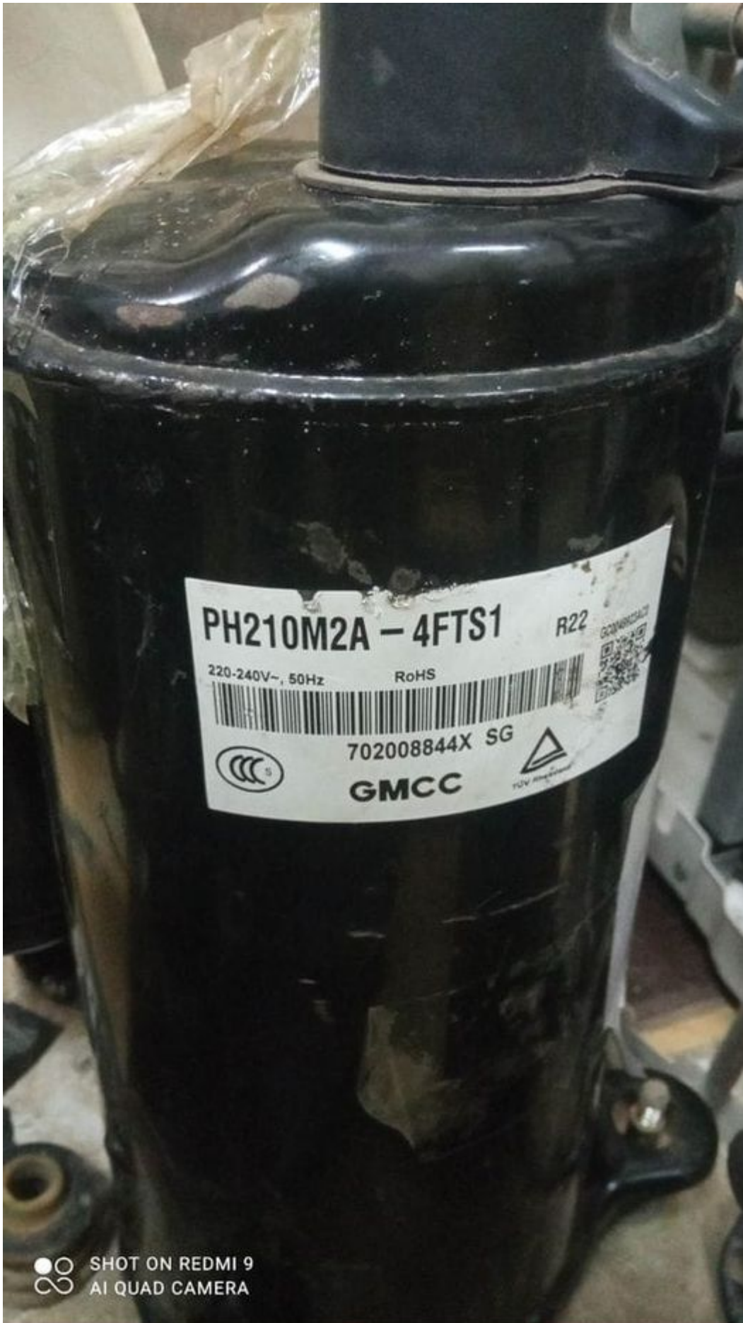
Mbsm.pro, PH210M2A-4FTS1, rotary compressor, GMCC, R22, 1.5 HP, 2.5 A.
