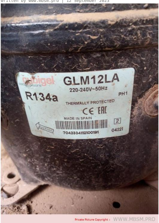
Mbsm.pro, Compressor, Cubigel/ACC, GLM12LA, R134A, 3/8 Hp, Lbp
