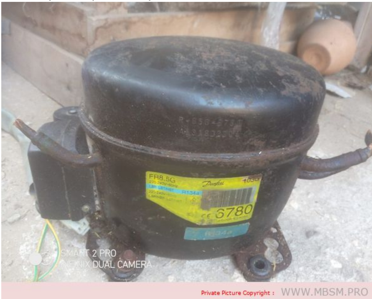
Compressor, danfoss, fr8.5g, 103g6780, 103g 6780, 1/4, LBP / HBP, r134a
