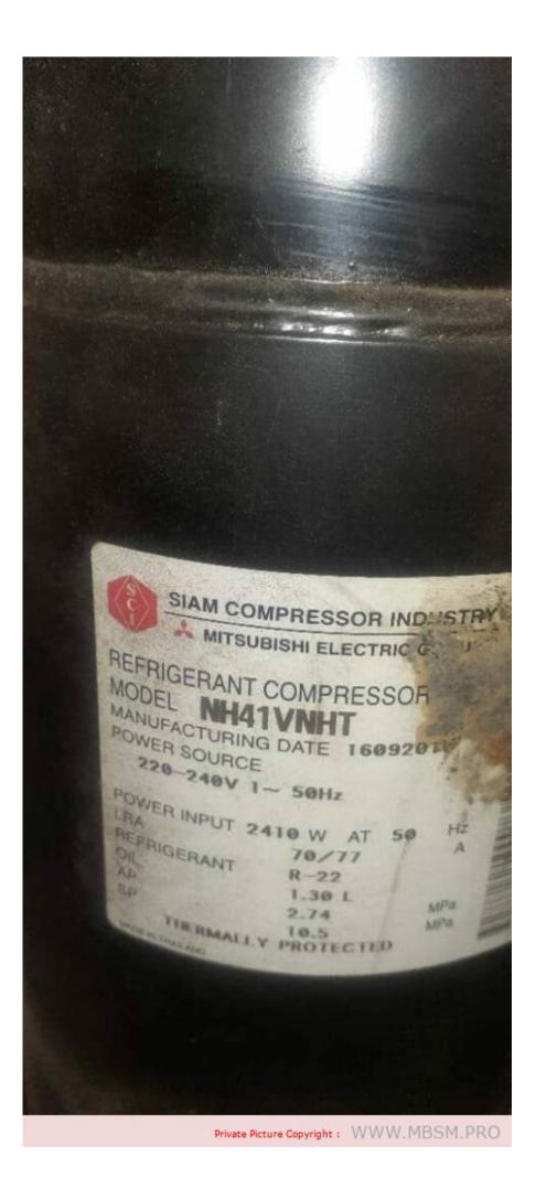
Mitsubishi, Electric, fixed frequency, NH41VNHT 2.55HP, single-phase, 220V, rotary, air condition, 26000 btu/h
