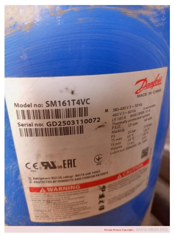
MBSM.pro, Compressor, 13HP, Danfoss, Performer, Scroll Compressor, Sm160, Sm161t4vc, Refrigeration Chiller, 3 ph, 380 v, 38BB 055 - 240, 38bb-250 9e/k, 38BB 250, 250 = 250000 kBtu/hr, 30 Ton, r22, 19 Kg, suction 1-1/8"-2, refoullement
