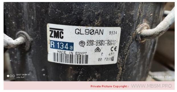
Mbsm.pro, Compresor, Danfoss, 1/4hp++, mhbp, Gl90an, R134a, 220-230v, 1ph, 50hz , Csir
