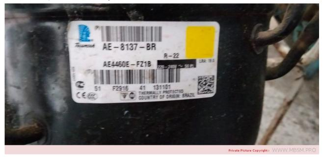
Mbsm.pro, Compressor, Tecumseh, AE4460E-FZ1B, 1/2 hp++, (big), r22, 220-240V / 50-60Hz, cold-room, chiller, AE-8137-br, 1421 w, 1222 kcal/h, 4846 btu/h, csir, hbp
