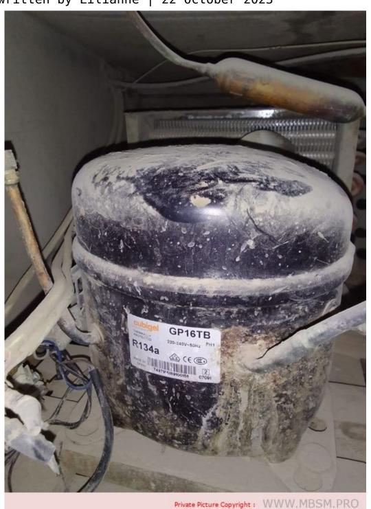
Mbsm.pro, Cubigel, GP16TB, hermetic, compressor, 3/8 hp++, 1/2 hp-, HBP, R134a, R1234yf, CSIR,
