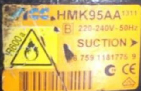
COMPRESSOR, DANFOSS, SECOP, HMK95AA, R600, 1/5CV, réfrigérateur , congélateur, LBP, Equivalent: EMBRACO NBM1114Y – NBM1116Y, DANFOSS NLE11KK – NL10K – NL11K – NLE15K, DANFOSS NLE11KK – NL10K – NL11K – NLE15K, DANFOSS NLE11KK – NL10K – NL11K – NLE15K, ELECTROLUX HP14AH – HP12AH, SECOP TLES8.7KK.3 – HMK95AA
