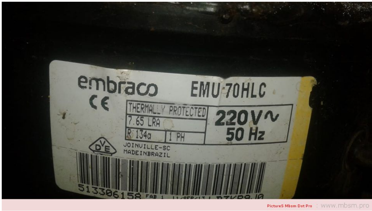
Compresseurs Embraco, ,EMU70HLC , R134a, 220 V, 50Hz, 1/5 HP, 149 watts , 0.17 kW (0.2214 BHP) ,180 mL
