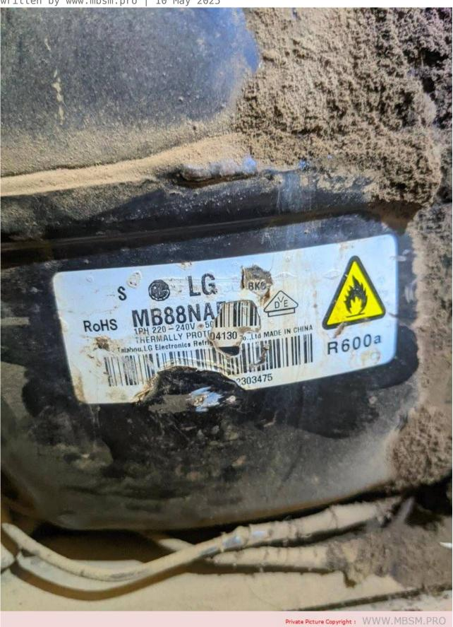
Mbsm.pro, Compressor, Lg, Lbp, MB88NA, 151 w, 1/5 hp, r600a, 1ph-220v-50hz
