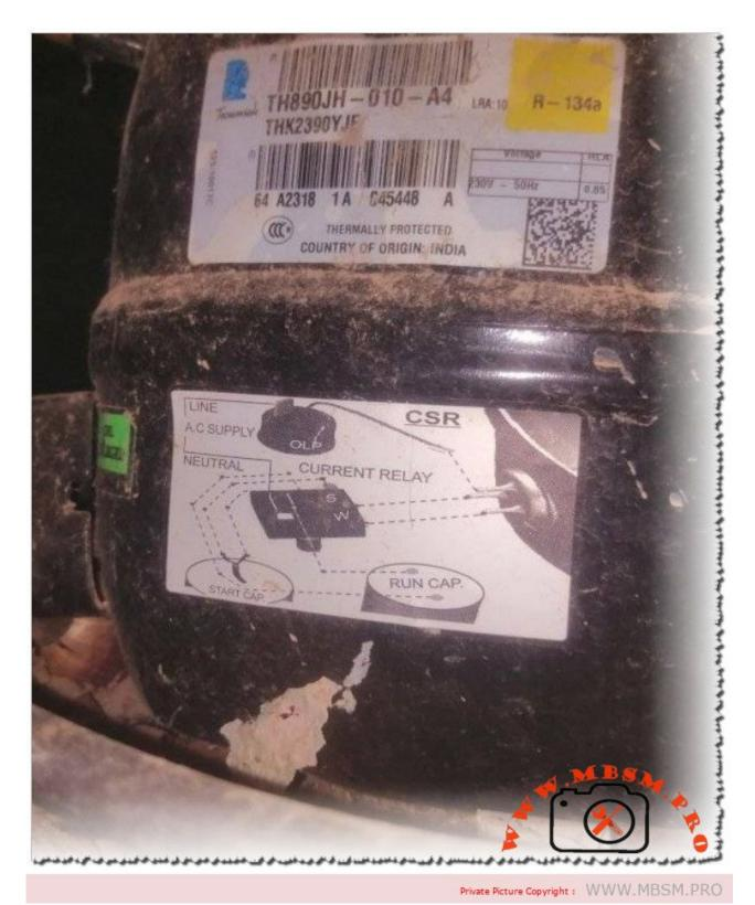
Mbsm.pro, Compressor, THK2390YJE, LBP, 1/3 hp, R134a, Freezing, Tecumseh Compressor
