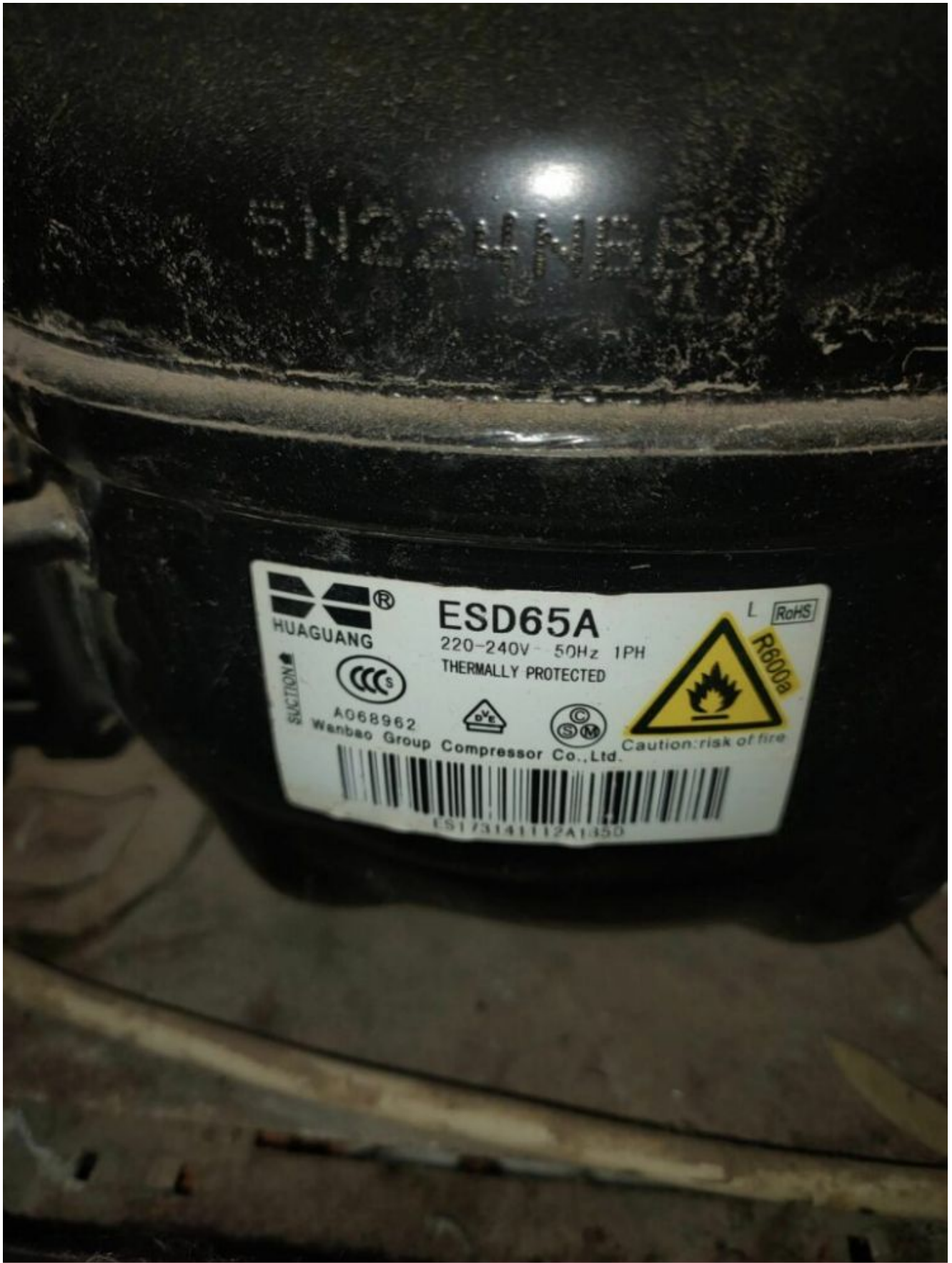
Mbsm.pro, Compressor, esd65a, 100 w, 1/8 hp, r600a
