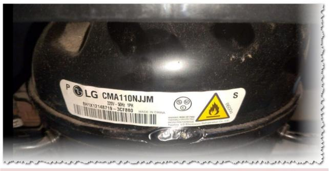
The LG CMA110NJJM compressor is a classic model that operates on a single phase with a voltage of 220V and a frequency of 50Hz. It boasts a fixed speed and is powered by a 1/4 HP motor. This compressor is perfect for applications requiring a steady and reliable performance.
