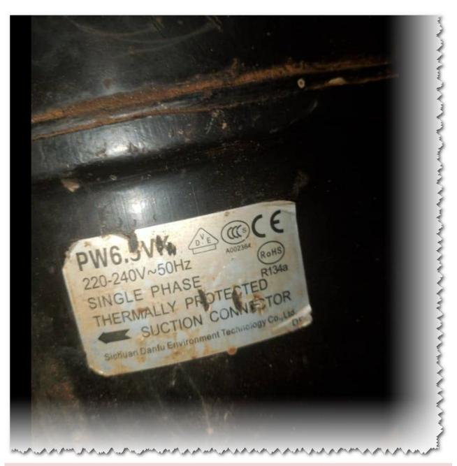
Mbsm.pro, Compressor, PW4.5VK, 1/8hP, 128 W, PW5.5VK, 1/6hP, 148 W, PW6.5VK, 1/5hP, 168 W, r134a, 1ph220v, watercooler, freezing
