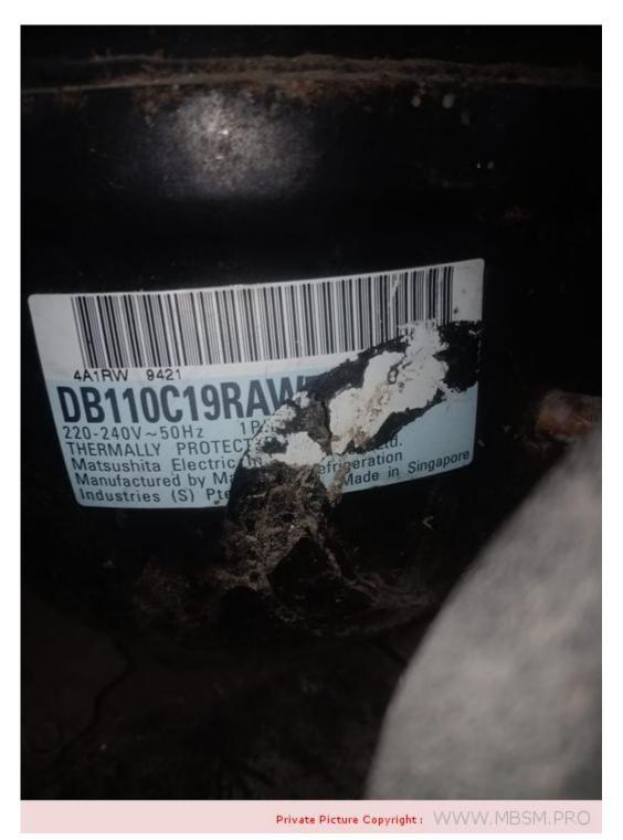
Mbsm.pro, Compressor, DB110C19RAW5, 1/3 hp, LBP, R134a, 200g, D series, Refrigerators, Smeg, 2 Doors, 18 feet, no-frost freezer
