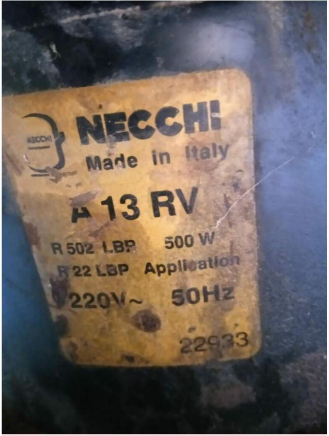
Mbsm.pro, Compressor, al3rv, 1/2 hp, Capacitor staring 53 to 64 mrf
