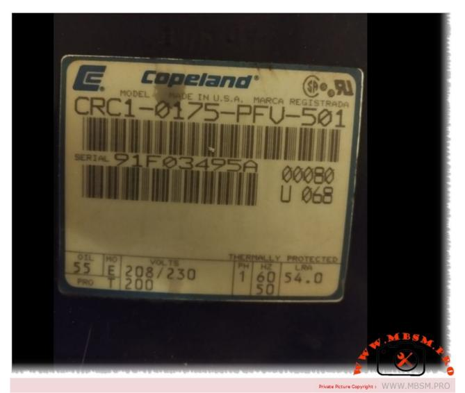
Mbsm.pro, Compressor, copeland, CRC1-0175-PFU-501, 2 ton, 2.25 hp, r22, compatible, ESAH-18CH, 18000 btu, 1920 w
