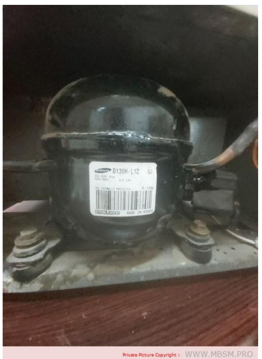
Refrigeration, Compressor, 1/10 HP, R-134A, Samsung, CD130C-L1Z2
