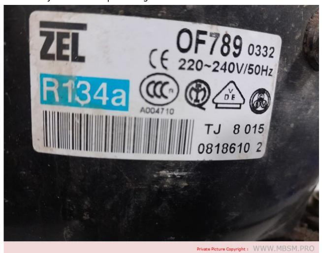
Mbsm.pro, Compressor, ZEL, piston, hermetic, compressor, P-0F789, GL45AA, AS45AA, OF789, GVY40AA, 1/8 hp, 106 w, r134 a
