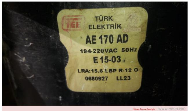
Mbsm.pro, Compressor, Tee compressor, ae170ad, ae170ac, ae170ap, 150 w, 1/5 hp, r12
