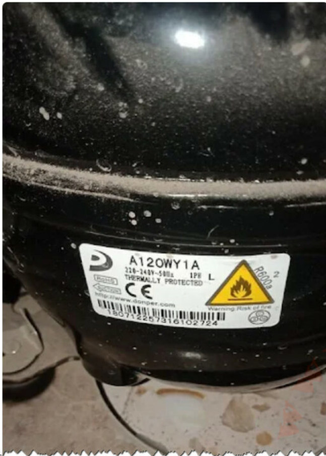
Mbsm.pro, Compressor, A120WY1A, 1/6 hp, r600a, Freezer, SONAX, 160 l, ES171-STANCARD, ES171STANCARD
