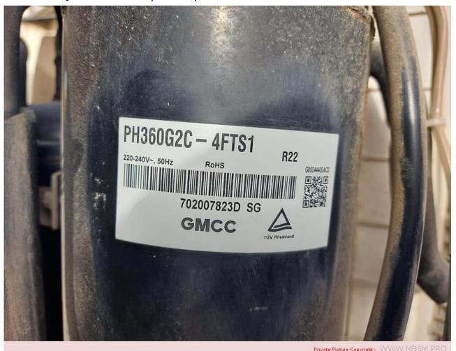
PH360G2C-4FTS1, 22000BTU, GMCC, Compressor rotary, air conditioner, R22, refrigeration compressor, 50HZ 220V / 240V
