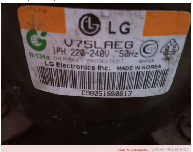
Compressor, LG, V75LAEG, V 75 Leag, 1/4 hp, 167 k/cal, 7.46 cc, 220v/50hz, Ptc, Rsir, compressor cooling, Lbp, r134a
