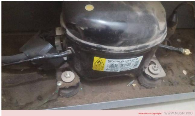
Mbsm.pro, Compressor, Refrigerator, GMCC, HITACHI, CL1588-Da, 1/5HP, R600a
