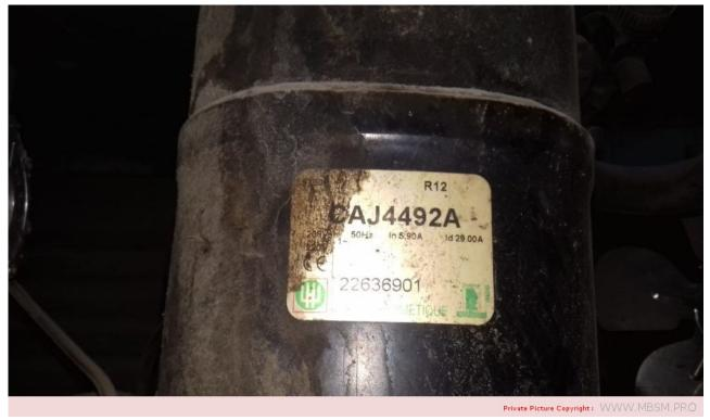
Caj4492A, R12, Tecumseh, Refrigeration, Compressor, 3/4HP, Medium/High Back Pressure
