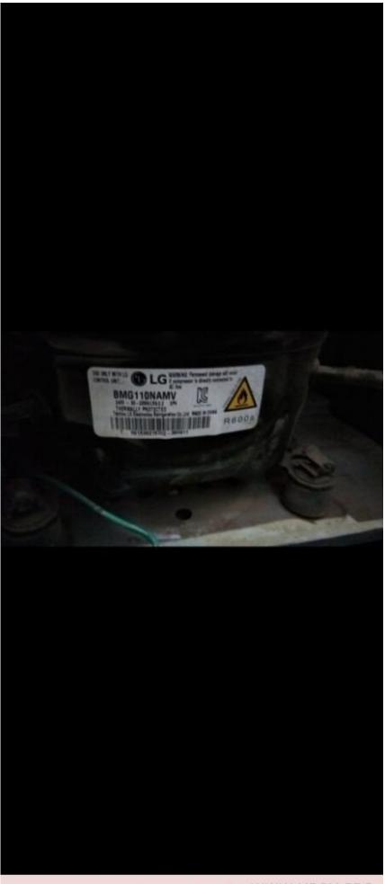
${\tt Mbsm.pro},$   ${\tt Compressor},$  inverter, LG Refrigerator, BMG110NHMV, BMG/BMA LG, Lbp, 1/4 Hp , R600A
