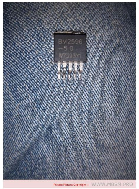
Mbsm.pro, BM2596, MSP1250G, 150kHz, 3A, Step-down, Voltage Converter
