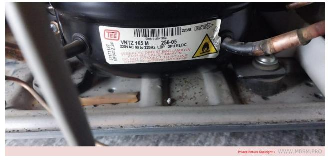
Mbsm.pro, Beko, Compressor, VNTZ165M, VNTZ165MT / VNTZ165M, Tee compressor, R600A, inverter, Blcd, 1/3 hp, lbp, Turk compressor
