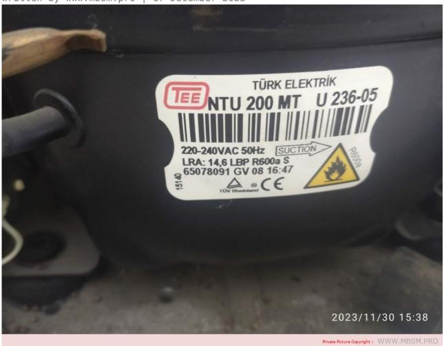
Mbsm.pro, Compressor, TEE compressor, Turk , 200 kcal, NTU200MT, 233 w, 1/3 hp, Lbp, r600a, lra 14.6A, Beko Compressor
