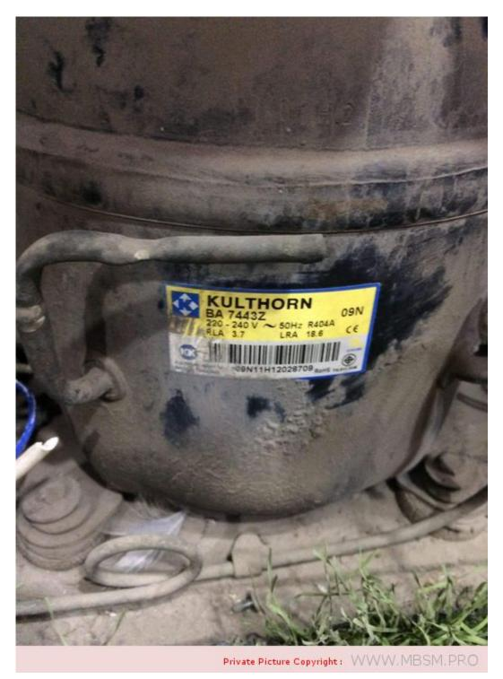
Mbsm.pro, Compressor, Kulthorn, BA Series, BA7443Z, 5/8 hp++, MHBP, R404A, 770 W, 3900 Btu, 1 hp-, 1 PH, 220 V
