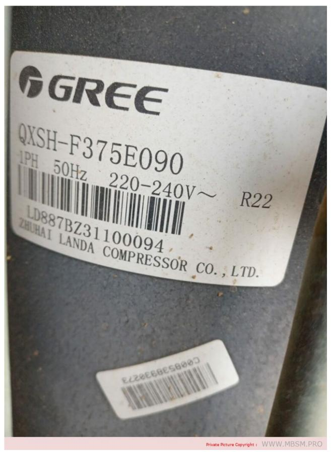
Mbsm.pro, compressor, Gree, Air conditioner, 0XSH-F375E090, 0XSH-F375, 22100 btu, 37.50 cm3, 6477 w, capasitor 60 uf, 1.8 ton, 2.8 hp, 220 v, 1ph
