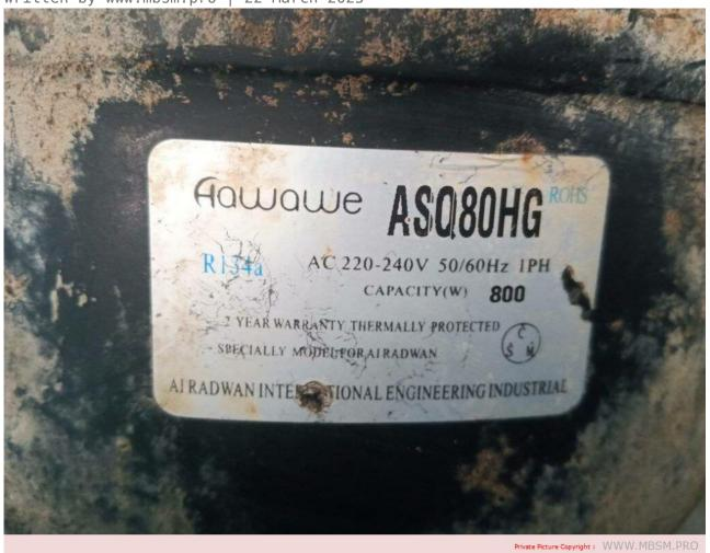
Mbsm.pro, Compressor, Huaguang, asq80hg, Q series, 800 w, Hbp, r134a, 1/4 hp, cooling Aplication
