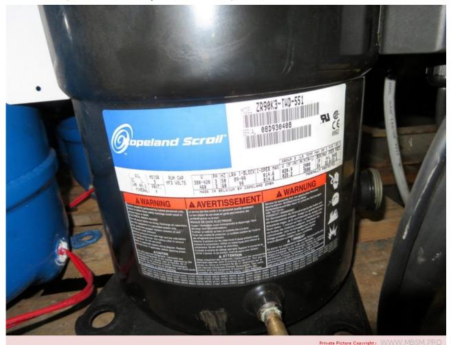
Mbsm.pro, Compressor, Copeland, ZR90K3-TWD-551, ZR90K3TWD551, 7.5 Hp, R22, 380-420/3/50Hz
