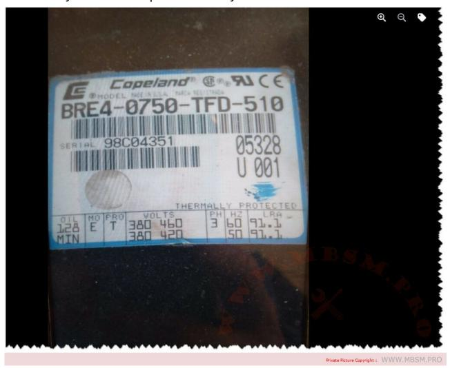
Mbsm.pro, compressor, BRE4-0750-TFD-510, Copeland, 7.5 HP, 460V, 3 PH, R22, R134A, R407C, Scroll Compressor, Copeland Compressor
