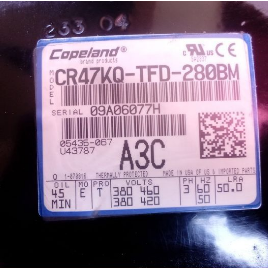
Private Picture Copyright : WWW.MBSM.PRO Mbsm.pro, Copeland, Hermetic, CR47KQ, Compressor, Series: CR, 47000 BTU/hr, 10.034 cfm, 460 VAC, 6.9 amp, 4 ton Tonnage, 60 Hz, 3 PH, 3500 rpm, 4 hp, 4540 watt, R-22, R-404A, R-407C
