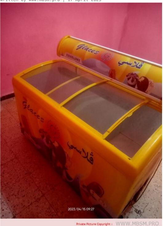
Mbsm.pro, Freezer, CF1441G, 210 L, Compressor, 1/4 hp++, 1/3 hp-, R134a, 145g, 370w, 220v
