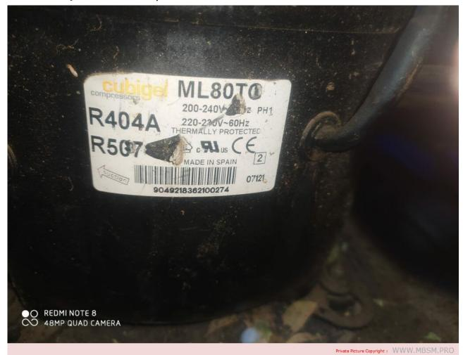
ACC, Compressor, Cubigel, ML80TG, 3/8 hp++, HMBP, 1/2 hp-, R404a / R507, 220-240V 50Hz
