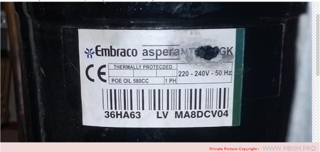
Mbsm.pro, Compressor, Embraco, Aspera, NT6220GK, Hermetic reciprocating compressor, R404a, MHBP, 17.4CC, 3/4Hp, ++big, 240V~50Hz
