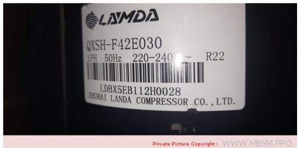
Mbsm.pro, Compressor, Gree, Rotary Compressors, QXSH-F42E030, 24000 BTU/HR, 2 ton, 3 Hp, 1PH / 220 v, r22
