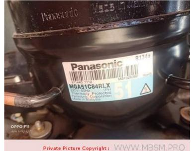
Mbsm.pro, Compressor, MGA51C84rLX, MGA51C68RPU, Panasonic compressor, M Series, Reciprocating Fixed Speed, 180 W, 1/5 Hp, RSCR, 220 V , r134a
