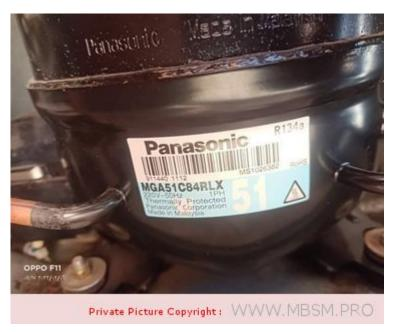
Mbsm.pro, Compressor, MGA51C84rLX, MGA51C68RPU, Panasonic compressor, M Series, Reciprocating Fixed Speed, 180 W, 1/5 Hp, RSCR, 220 V , r134a
