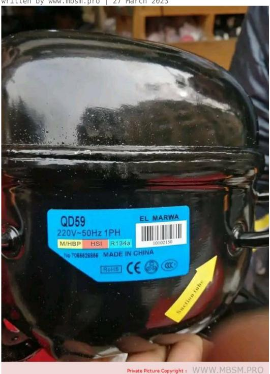
Mbsm.pro, Compressor, Qd59, 1/6 hp++, 1/5 hp-, 142 w, QD series Compressor
