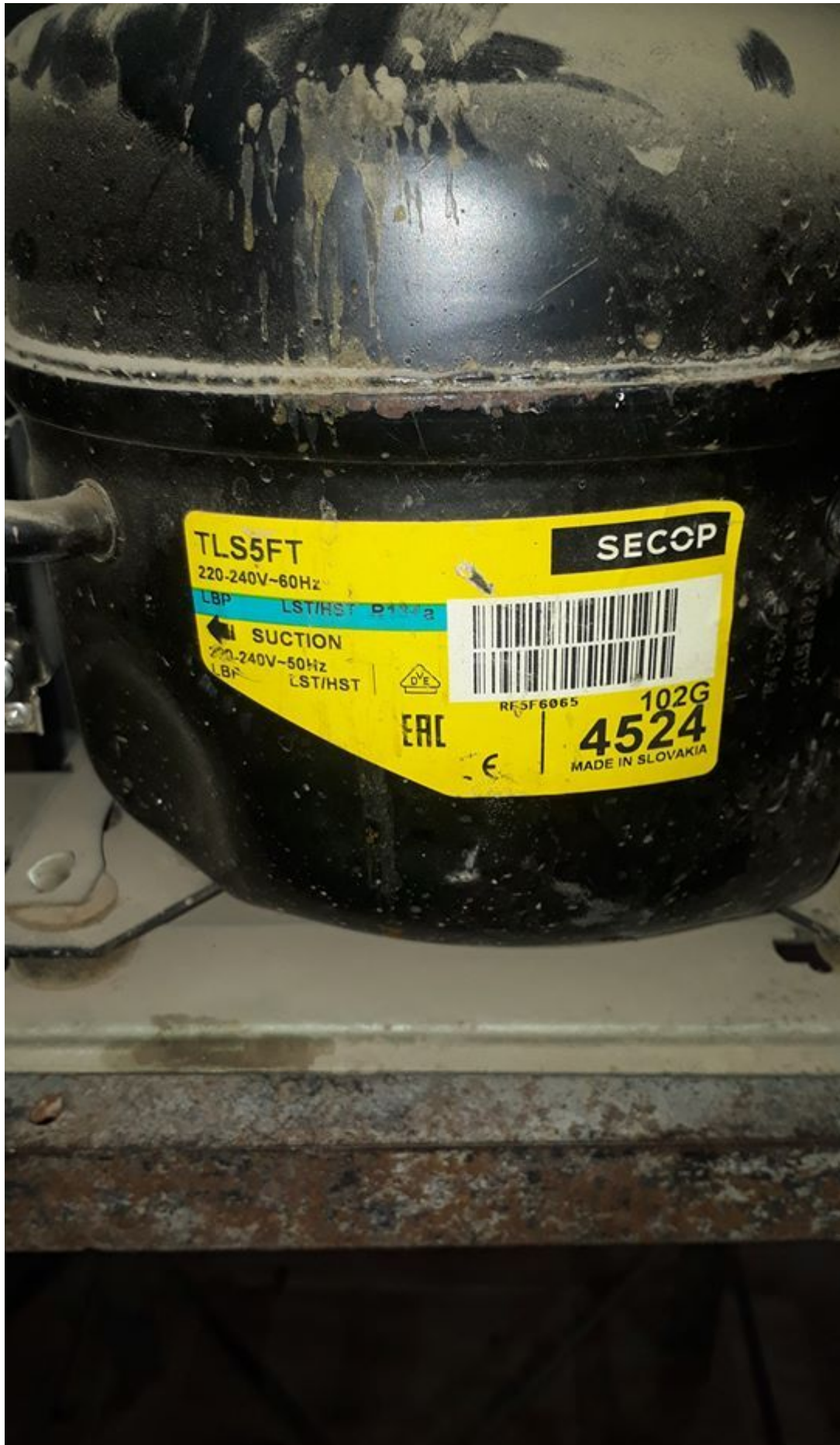
Tropical Compressor ,TLS5FT 102G4524 , SECOP , R134a , 1/6 HP , 134 W , LBP , 220/ 240 V 50Hz
