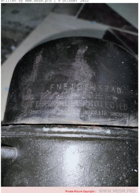
Mbsm.pro, Compressor, r12, 1/6 hp, 125 w, FNE125W, fne125ws7ad, fne125ws, 230V/50HZ
