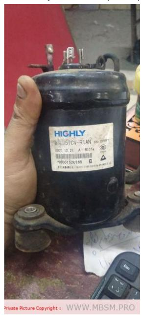
Mbsm.pro, Compressor, bsa357cv-rlan, Highly, Hitachi, R134a, Rotary Compressor, for Air Condition, 220/240V, 1245BTU, run capacitor 5 mF/38, replaced by qx36h
