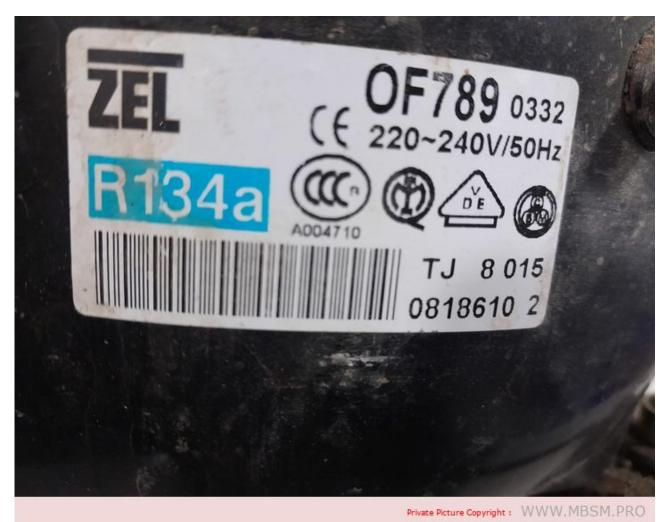
Mbsm.pro, Compressor, ZEL, piston, hermetic, compressor, P-0F789, GL45AA, AS45AA, 0F789, GVY40AA,1/8 hp, 106 w, r134 a
