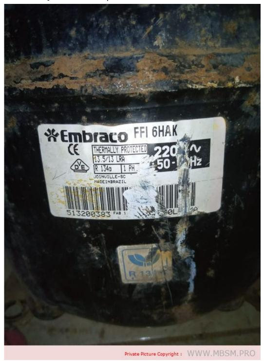
Mbsm.pro, Compressor, Embraco, 1/5hp, Ffi 6 Hak, Ffi6Hak, Ffi6 Hak, Ffi 6Hak, FfI 6 Hak, R-134a, 220v Mbsm.pro, Compressor, R134a, FR7.5G, 103G6680, 220-240V 50/60Hz, LBP/HBP, 1/5HP++, 1/4 hp-
