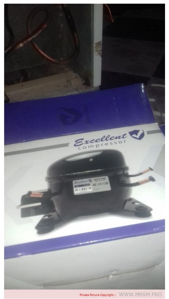
Mbsm.pro, Compressor, gs77af, 1/5 hp, lbp, replacement, GL70Ah
