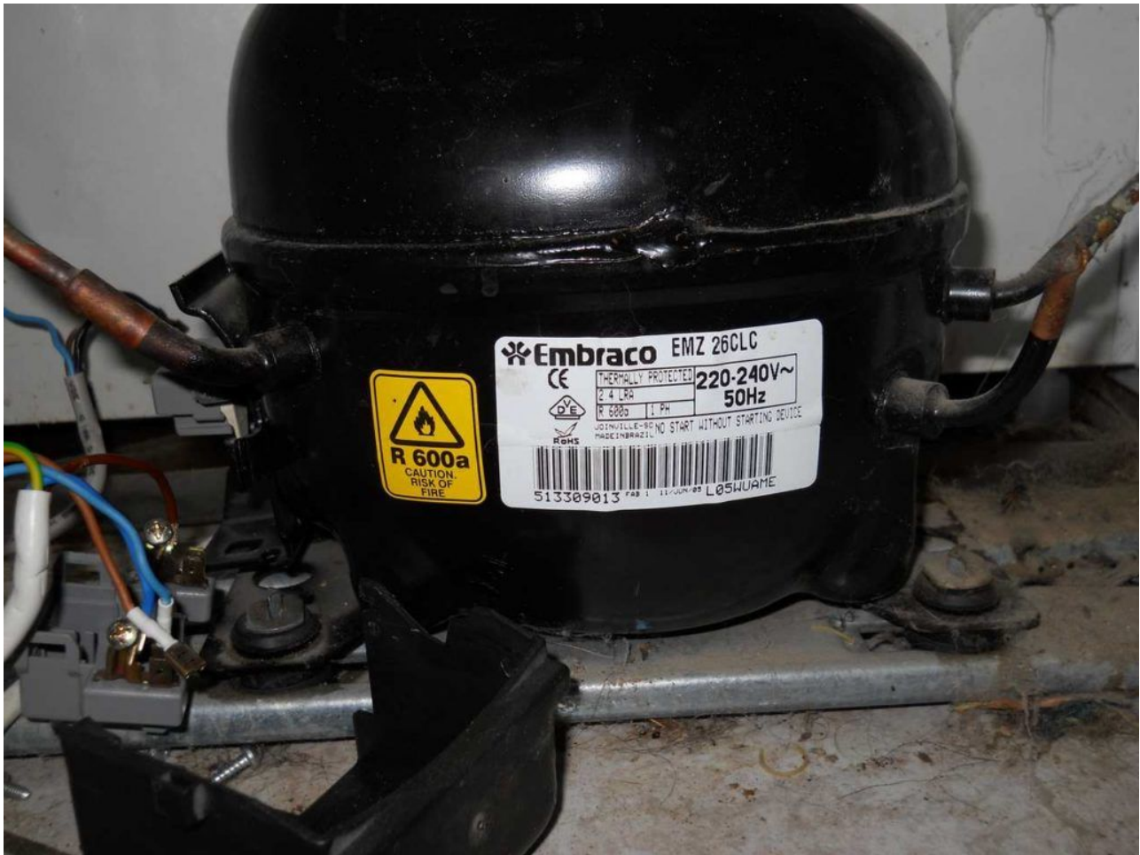
Compressor, Embraco, Aspera, EMY26CLC, LBP, R600a, 220 – 240V/1/50Hz, 1/12 HP, RSIR, LRA 7.8 A, 83 Wat
