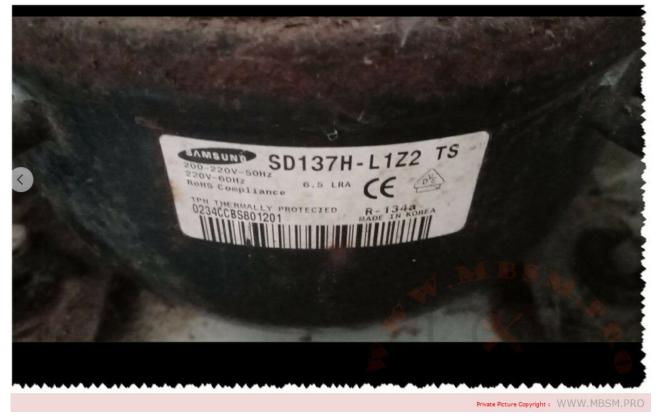
Mbsm.pro, Refrigerator, Compressor, SD137H-L1Z2, 1/10hp, lbp, r134a, lph, 220v/50hz
